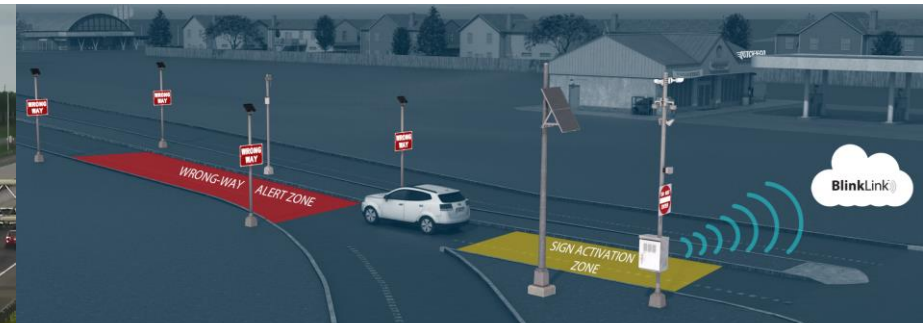
Wrong-Way Driving Detection System
